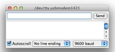
The code uses **Serial.begin(9600)** to open a serial connection back to your computer in setup(), and **Serial.println(...)** to output ("print") numbers to that serial connection, which end up in the Serial Monitor window on your screen. It's also possible to send data back to the Arduino that way, using **Serial.read(...).**
