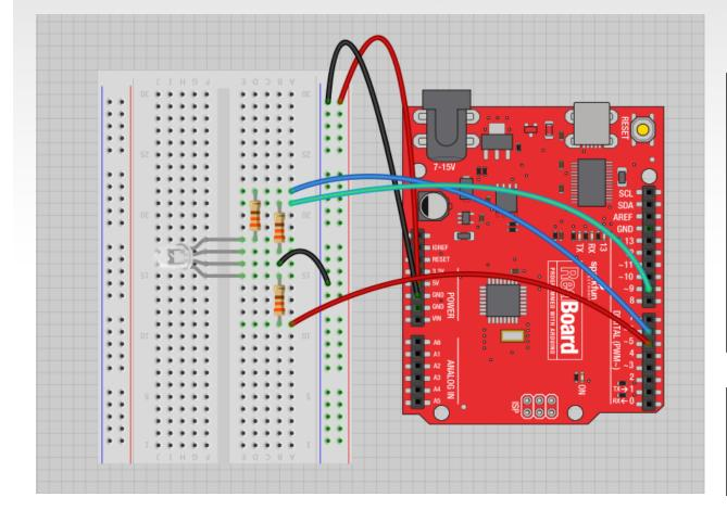
Note: The longest leg of the RGB LED is the Common Cathode. This goes to GND.
