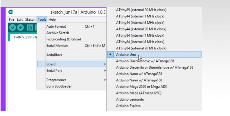
Next, double-check that the proper board is selected under the Tools $\rightarrow$ Board menu.
