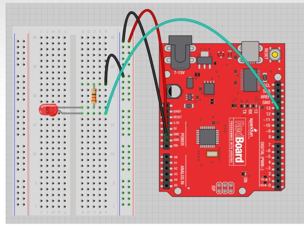
Move the green wire from the power bus to <u>pin</u> <u>13 (or any other</u> Digital I/O pin on the Arduino board.
