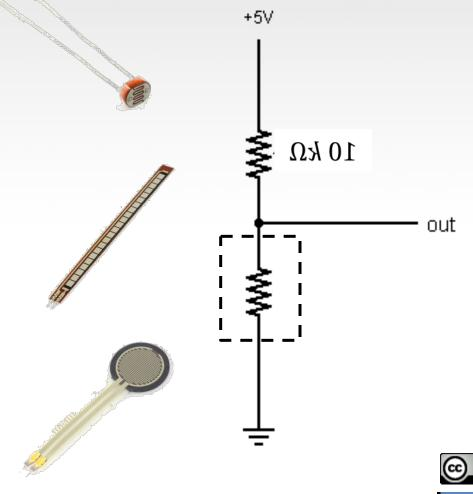
Take two sensors -- Use the Serial Monitor and find the range of input values you get for each sensor.
